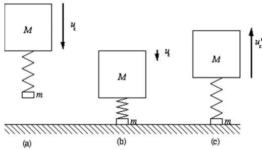
**Fig. 3** Dynamic effect of a foot, mass  $m$ , connected to the remainder of the system  $M$  by a spring. The energy lost each stance is  $mv_z^2/2$ , where  $v_z$  is the vertical component of system velocity.
