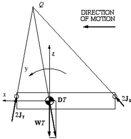
Fig. 1 Impulsive equilibrium over the duration of a stride for a bound.  $W$  is the weight of the system, and  $D$  is the drag.  $T$  is the stride duration.  $2J_F$  is the net impulse imparted by the front feet, and  $2J_R$  is that imparted by the rear feet.
