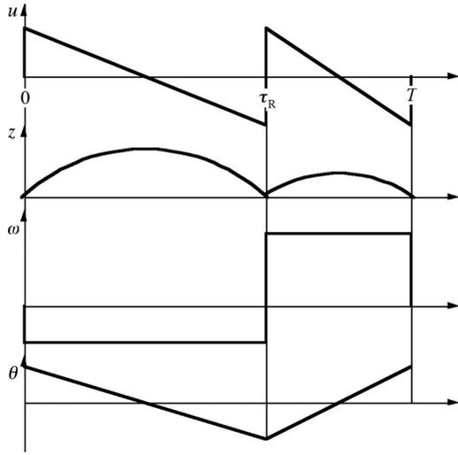
**Fig. 6** Variations in vertical velocity and vertical position of center of mass, and pitch angular velocity and pitch angle through a bound stride. The intervals used in the text are  $\tau_{FR} = \tau_R$  and  $\tau_{RF} = T - \tau_R$ .
