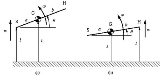
Fig. 5 Coordinate senses during the (a) front foot stance, and (b) rear foot stance. Point S represents the shoulder joint, and point H represents the hip joint. G is the center of mass.
