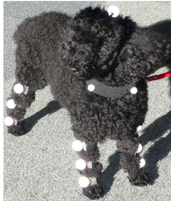
Fig. 2. A subject as outfitted with a simplified passive reflective markers set with three on each leg, a four around the collar, and one on the head.
