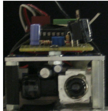
Figure 1. The Stanford SLASR adds a diode laser, aspherical camera lens, and tuned filtering circuitry to the Sharp GP2Y0A02YK sensor
