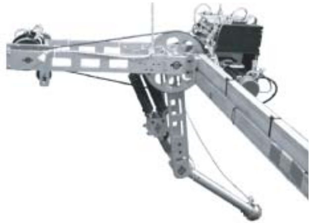
Fig. 2. The OSU DASH leg, attached to test boom.
