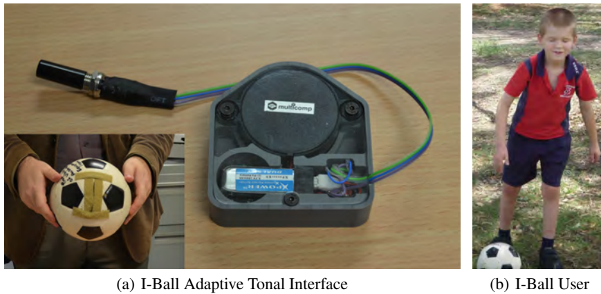
Fig. 1. (a) The I-ball features a smart embedded circuit, a rechargeable battery, and a gyro to provide an adaptive tonal assistance (in inset: ball with circuit installed). (b) A child with total vision impairment playing soccer using the I-ball
