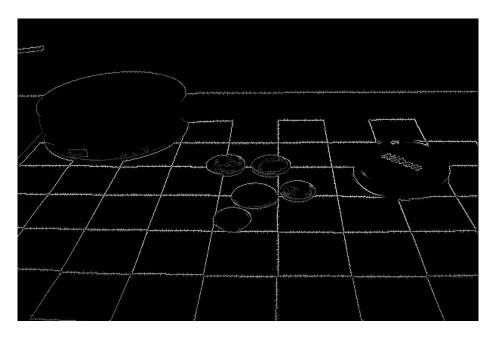
Figure 1: chess\_circles.jpg after Canny edge detection
