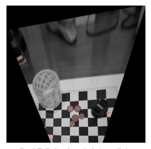
Figure 2: The Hough transform results after image rectification
