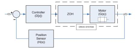
Eliza has selected a **1 kHz sample rate** for the digital controller and has characterised the turntable and sensor as:  $G(s) = \frac{5}{s(s+20)}$  and H(s) = 1.
