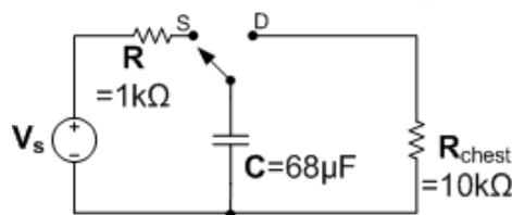
With the switch in the standby mode ("S"), the  $68\mu\text{F}$  capacitor is charged using a controller (having a Thevenin equivalent of  $V_s$  and  $R=1\text{k}\Omega$ ). To defibrillate, the switch is thrown (to "D") and the capacitor discharges across the patient's chest, which can be approximated as a  $10\text{k}\Omega$  resistor.
