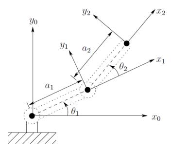
Figure 1: Two-link Planar Robot
