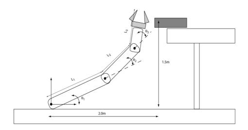
Consider the three link arm below in a <u>vertical configuration relative to gravity</u> (i.e., Gravity is pointing into the from the top of the page to the bottom or  $g=[0\ 0\ -9.8]\ m/s^2$ )
